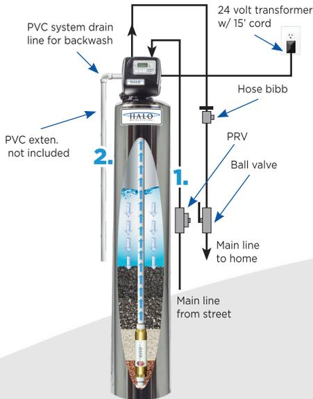
1. Plumb inlet/outlet to system main.
