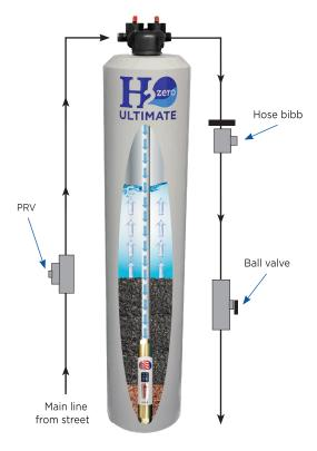
Installation of a hose bib and a shut off (ball valve) is required downstream from the unit.
