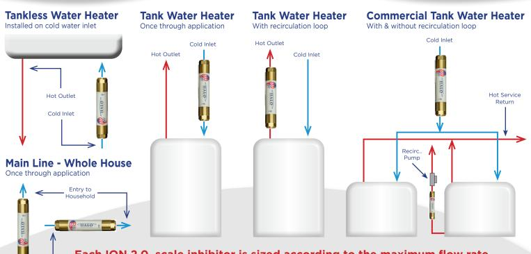
Each ION 2.0 scale inhibitor is sized according to the maximum flow rate at which it will condition the water most effectively. The HALO ION Scale Inhibitor does not restrict water flow\*
