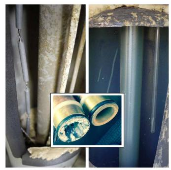
WITHOUT TREATMENT After nearly 7 years of service on San Diego Municipal Water with no water treatment installed. Accumulation of Scale & Corrosion WITH HALO ION After nearly 7 years of service on San Diego Municipal Water with HALO 5 (INCLUBES 100) water treatment installed. NO EVIDENCE OF SCALE OR CORROSION (The marks on the back wall of the heater are where we ran a fingertip along the back to demonstrate the presence of the Argonite taic.)
