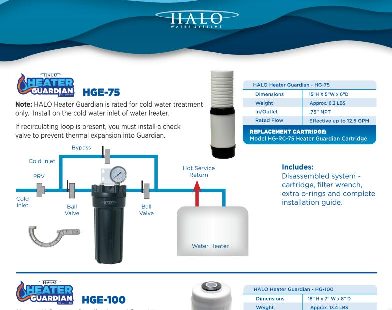
**Note:** HALO Heater Guardian is rated for cold water treatment only. Install on the cold water inlet of water heater.
