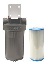
5 micron sediment filter reduces sediment, sand, silt, scale and rust particles. Pleated design maximizes sediment holding capacity.
