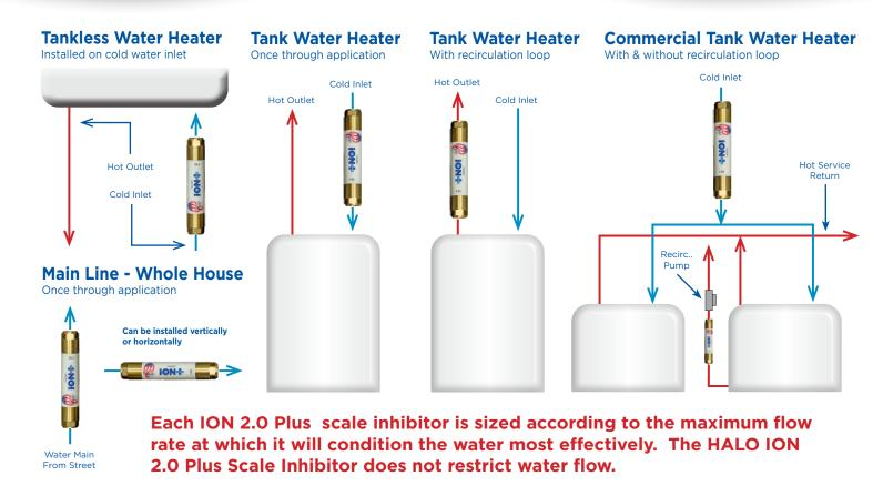
**PRO TIP:** The newly designed HALO ION 2.0 Plus no longer needs dielectric unions unless dissimilar metals are present to ensure electrolysis is not an issue during soldering.
