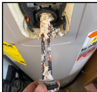
Severely Scaled Heating Element
