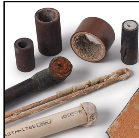
Scale buildup in various plumbing pipes (before ION was installed)
